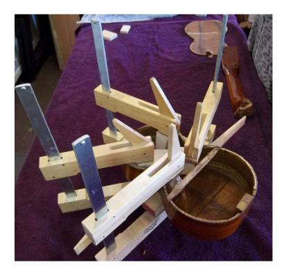
The first thing I needed to do was to re-glue the two top braces. As I thought, this flattened the top quite well. I used a PVA glue, not hide glue, on this repair, since I wanted the braces to attach more firmly to the top.
