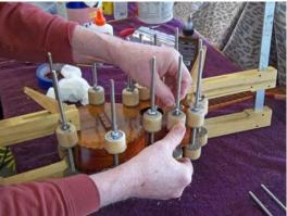
Now that I was satisfied with the neck joint, it was time to reattach the top. Again, I applied hide glue to the top of the sides and the kerf lining, then clampled the top in place.
