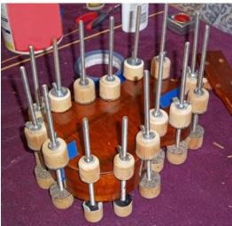
Now that all the cracks have been repaired, it was time to glue on the back. For this type of repair I do use hide glue. I use a pre-mixed liquid version of hide glue that's available at hardware stores. Hide glue is reversible, which means with a little heat and/or moisture, it becomes tacky again. This is great when tops and/or backs need removing for repairs.
