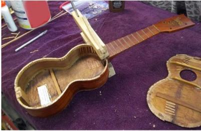
The neck's dovetail joint has slots on both sides that the thin side pieces of the uke fit into. I had to first clean out the slots since pieces that broke from the body were still glued inside.
