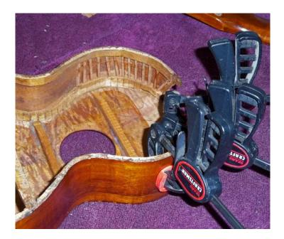
For several days, I continued to make and glue the thin strips of wood on the inside over the cracks. As you can see in the photo, I made the strips run from kerf to kerf.
