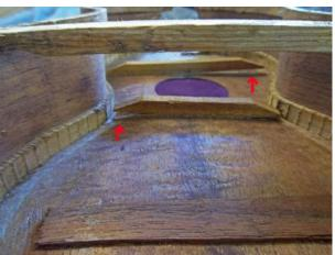
On Day 2, I removed the back. Recently I acquired a specialty heating device that included a type of matte knife that attached to the end. This is basically a wood burning tool, but it came with several attachments for different types of work. It has a rheostat I can set from warm to very hot. For the old hide glue, I ran a damp sponge around the edges already loose, then set the burner on warm, and slowly ran the knife around the edges. Within an hour, the back was off.
