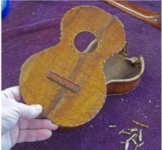
Now that all the cracks have been repaired I needed to take off the top so I could remount the neck.
