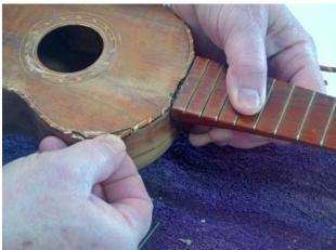
Before putting the pieces of rope binding back on, I had to first clean the channels. The hide glue had squeezed out onto these small edges, so I had to use a micro chisel to scrape it. Cleaning took a couple of hours on Day 17.
