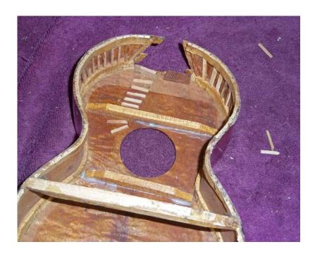
Because the top had warped so much from the loose braces, a hairline crack had developed just below the opening where the neck goes. I injected a little PVA glue into the crack, and then, after it dried, added a few thin cleats to strengthen the area.
