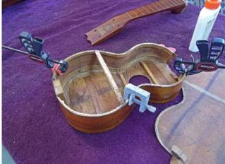
Now that the side cracks were closed I started gluing thin strips of wood (cleats) on the inside to strengthen the sides and to keep the cracks from opening again.
