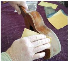
When I put the top back on, I was able to get most of the squeezed-out glue cleaned off, but with all the clamps in place I couldn't get at all of it. Today I used a cabinet scraper to get the remaining glue off, then sanded down the surfaces with sandpaper to even out the finish around the repairs.
