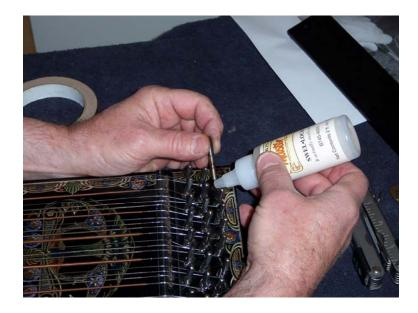
Often when removing zither tuning pins, the holes seems to expand. When reinstalling the pins, several often don't have the friction to hold a tightened strings. There is an interesting liquid product called Swellock, that can actually swell the wood to make parts fit tighter. It's usually used on chair tenons to tighten loose joints, but I've been able to use it on tuning pin holes to make the pins fit tighter.
