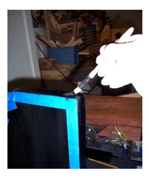
With the back finished, I needed to touch up the sides where I had closed up the failed glue joints. The sides originally had a glossy finish, just like the tail pin cover, so I used the same glossy black enamel to recoat and touch up the sides. This was another three coat, three day project.
