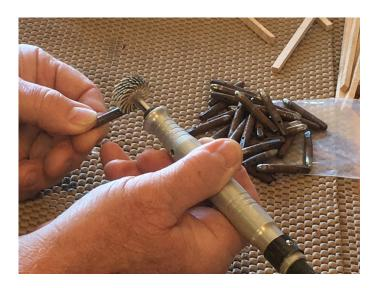
The tuning pins were quite corroded and needed a lot of cleaning. This is a time-consuming process. To clean them, I use one of my rotary carving tools with a fine (120 grit) flap sander. It took nearly three hours to clean the 32 pins.
