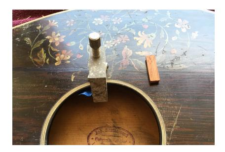
I wanted to make sure the top crack would be very stable, so I glued a couple of cleats, small, thin pieces of hardwood, to the underside of the crack.
