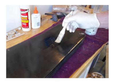
Now that the patching is done, and I've cleaned all the dust off with a tack cloth, I can paint the back. For the next three days I put three coats of a satin (not glossy) black on the back. It seems most zithers, both concert zithers and chord zithers, have backs painted a satin or flat paint, while the sides are often a glossy black. More ornate concert zithers more often have wood veneered sides to match the top veneer.
