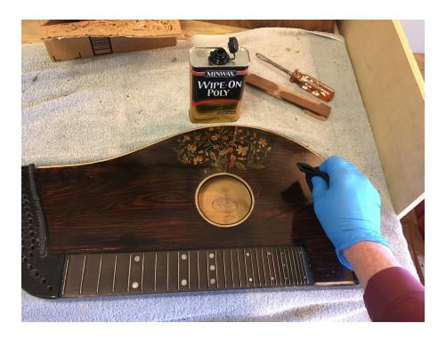
After the stain was quite dry, I used a clear wipe-on poly to seal the top. This polyurethane is like the original lacquer but a bit safer to use.
