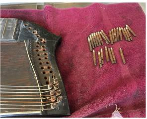
On Day 2 I removed the strings. As I mentioned before, the strings were in quite good shape. As I removed the strings one-by-one, I wrapped a piece of tape with the string type and number. I marked the first 12 melody strings with M-1, M-2, etc. The 12 bass strings were marked B-1, B-2, etc. Contrabass, CB-1, etc.
