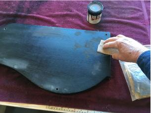
The back also needed a little patching to fill some small gouges and scratches. For all the patching I do to small blemishes I use a special water-based ebony filler. It dries quite hard and doesn't shrink or peel like many commercial non-water-based fillers found in hardware stores. The filler I use comes in many colors, so I can use whichever color suits the wood I'm working on. Ebony works best here because all the side and back surfaces are black.
