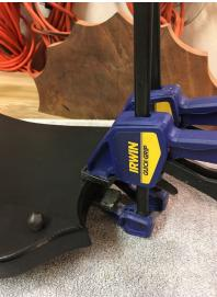
An ugly problem arose after I string up the zither. The top had pulled away from the side. This problem probably existed before but must have been closed enough so that I hadn't noticed it. With the strings tightened, the opening was more pronounced.
