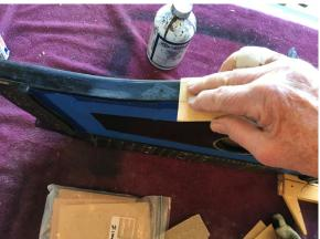
To prepare the zither for staining and painting, I lined the top with painter's tape so no paints would get on the rosewood veneer top.
