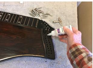
Another laborious part of the restoration process is reinstalling the tuning pins. Often when pins are removed the holes seem to dry more and expand just enough that the pins won't hold the string tension.
