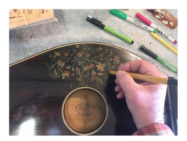
Where the top crack was previously fixed by someone else, the narrow glue and patch job ran through the decal, blotting out portions of it. Also, the decal had a couple of small pieces rubbed off from years of use.
