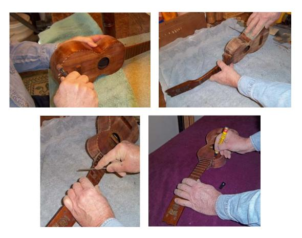
Today, I used a small rotary sander to even out the rope binding, then did a final sanding, going through several grades of sandpaper, from 180 grit to 600 grit, finishing with 0000 steel wool.
