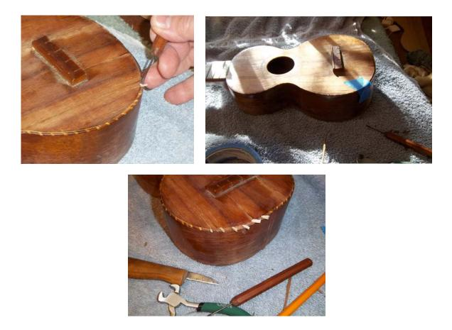
For the next three days, I cut and glued tiny pieces of koa and maple to replace the missing section of rope binding. I could only glue one piece at a time, and wait for it to dry before adding another piece.
