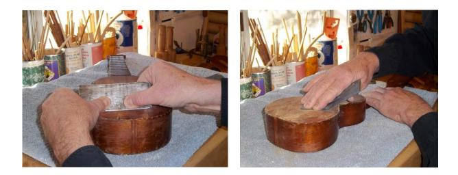
Now that the ukulele is together, I needed to scrape the instrument to take off glue that had squeezed out from the clamping process. Because scraping takes the old finish off, I needed to sand most of the uke to even out the surface so later touch-ups wouldn't look uneven and blotchy.
