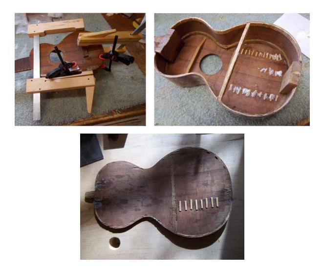
This day I did quite a bit of work on crack repairs. After injecting glue into the cracks, I put pressure on the sides of the top using a cam clamp to close them up. I used the other clamps to keep the top from buckling under pressure.
