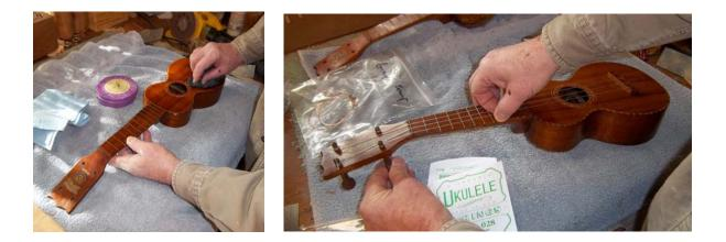
A few days later, after the varnish dried fully, I added a little extra protection with a nonabrasive paste wax. I applied it using very fine 0000 steel wool soaked in the wax. Using steel wool instead of a cloth keeps the original matte look and doesn't polish the uke to a high gloss.
