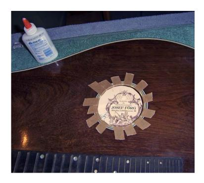
The sound hole binding was the biggest problem. The old plastic had shrunk and pulled away from the wood. After gluing it back in, there was a small gap left that I'd have to fill with some matching plastic.
