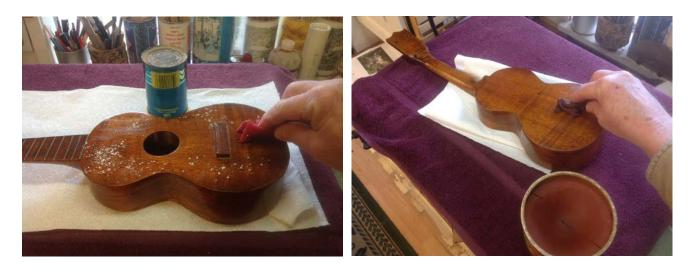
Kumalae ukuleles were originally finished with a French polish. French polishing is a wood finishing technique that results in a high gloss surface. French polishing consists of applying many thin coats of shellac dissolved in alcohol using a rubbing pad lubricated with mineral oil.
