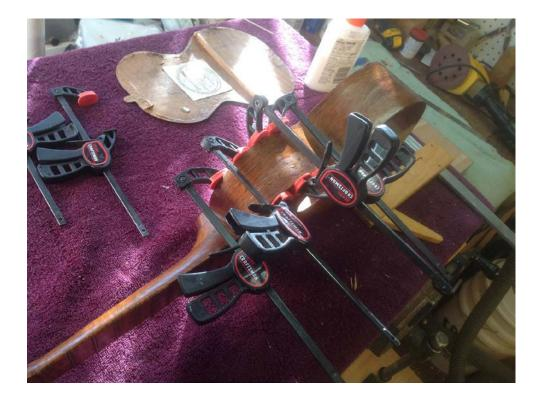
For the next two days I continued working on the side cracks. Because cracks were present most of the way around the sides, I had to work on one section at a time. The types of clamps I use do not use a lot of force. With the sides so thin, around 1/16 of an inch thick, heavy clamping would crush the wood. These small bar clamps are perfect.
