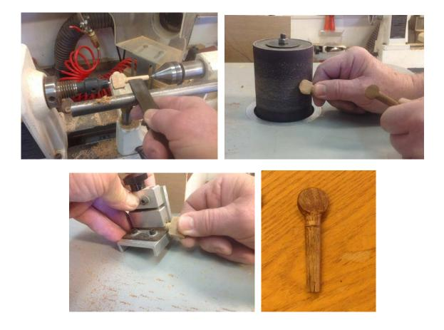
I took a break from the side repairs this day and made a replacement for the missing tuning peg. The original tuning pegs are a wood I couldn't identify. They aren't koa, but probably another Hawaiian hardwood.
