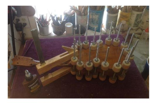
Now with the top and sides repaired, it was time to glue on the back.
