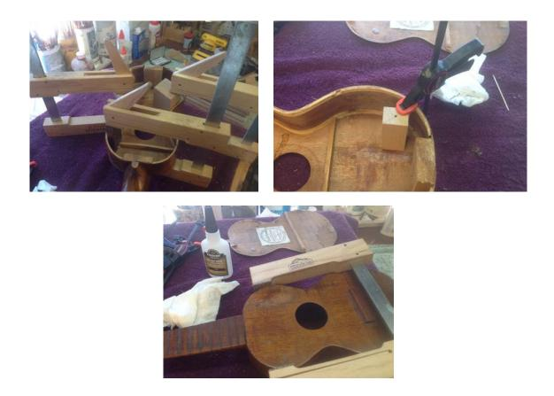
Early in the day I repaired the loose top braces by forcing glue under the loose areas and clamping them down. Not only did this fix the loose braces, but it also leveled the top. With loose bracing, the top had a slight "wave" to it.
