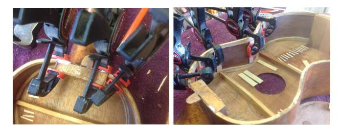
The sides of the ukulele, where they attach to the neck block, were loose. The old hide glue had failed. I cleaned as much of the old hide glue off as I could and forced new hide glue into the joint.
