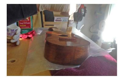
Each day, for several days, I brushed and rubbed on a tung oil varnish. Each coat needed 24 hours to dry before putting on the next coat.
