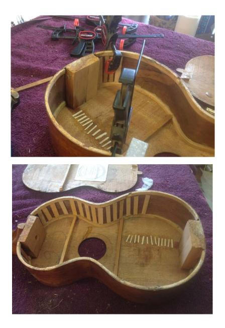
For the next couple of days, I continued gluing the thin cleats to the sides.
