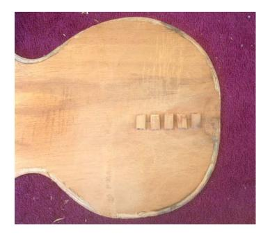
After the glue in the crack dried, I made up some thin cleats of scrap koa and glued them across the length of the crack.
