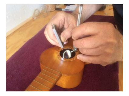
Before continuing work on this ukulele, I did an interior inspection to see if there were any maker's marks, numbering, or damages.
