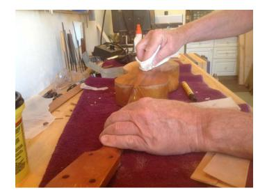
After a final sanding with 0000 steel wool, I cleaned off the uke with a tack cloth and began applying a stain that matched the original, a light oak stain.
