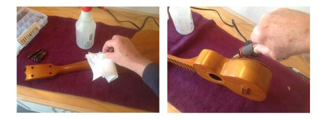
To do a good repair on the back crack and to be able to stabilize it well, I removed the back.
