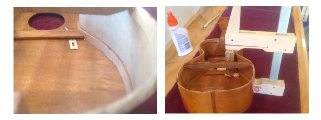
With the back off, I noticed a slight gap in one of the top braces. I slipped an Xacto blade under to see how much of the brace had come loose.
