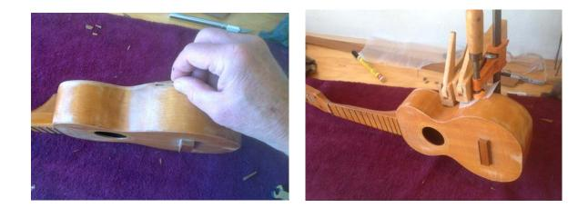
To fix the small crack where the back brace was pushing into the side, I opened it a little and cut into the brace a little with a micro chisel so I could place and glue a small piece of matching koa into the opening.
