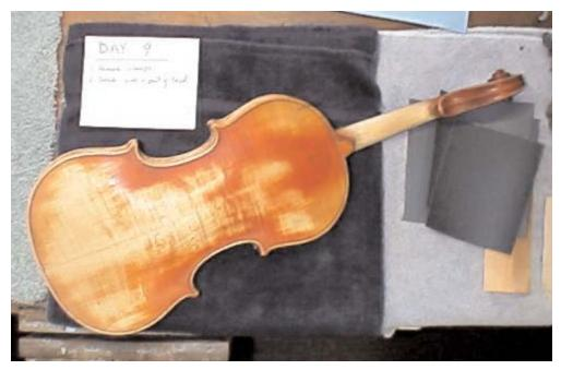
After removing the clamps, I sanded down the front, sides, and back once more. I refrained from removing all the previous finish on the back because I didn't want to disturb the stamped in maker's mark at the base of the neck. There were a couple of "gouges" in the back that I sanded down, and I planned to match and blend in the varnish as best as possible.
