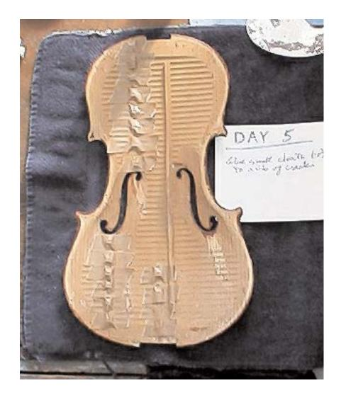
When a string instrument has a large top crack, it's common to glue tiny cleats on the inside to add strength to the seam. I used small pine pieces and set them in with the grain running perpendicular to the top.
