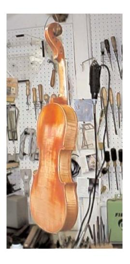
Because I completely removed the top varnish, the violin needed a sealer coat before applying the red spirit varnish. I used a red oil varnish as a sealer, which soaked into the bare top wood nicely.
