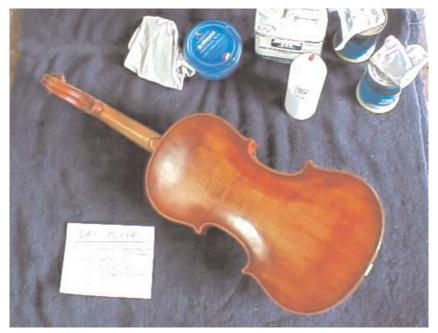
Day 13 saw us in a warm spell. The rains stopped again, and I was able to apply the last coat of varnish, which only took one day to cure (instead of three or four). On Day 14 I began the rubbing out process, using mineral oil soaked rags coated with pumice and rottenstone. These are light abrasives that smooth out the brush marks and the inevitable dust specks. I also fabricated a nut and glued it and the saddle in place.
