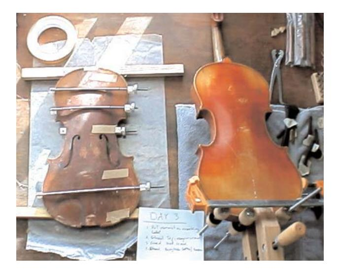
Day 3 was exciting. The large top crack was a clean break and clamped together quite easily. The specially curved violin clamps I used kept the top from bowing in or out. The back seam crack and the space between the back and sides where the glue had failed took a little more effort. These areas were filled with years of dust and dirt, as well as "chunks" of hide glue, and required a thorough cleaning before I could glue them.
